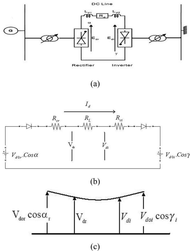
Figure 3. (a) One line diagram, (b) equivalent circuit diagram and (c) voltage profile on a monopole HVDC system
