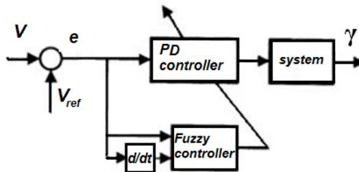
Figure 5. Inverter control system (PD & FUZZY)
