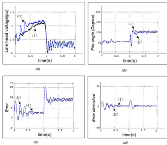
Figure 12. Comparison of performances of PD and Fuzzy-PD controllers; a: line head voltage; b: fire angle; c: error; d: error derivative; (I: Fuzzy-PD controller on rectifier and PD controller on inverter; II: Fuzzy-PD controller on both converters)
