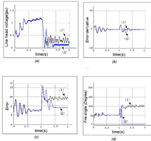
Figure 16. Performance comparison of Fuzzy-PD controller on both converters with three phase fault on load; a: line head voltage; b: error derivative; c: error; d: fire angle; (I: controller working continually; II: line power is disconnected when fault isn't removed)
