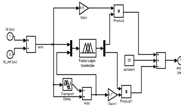
Figure 8. PD-Fuzzy rectifier controller
