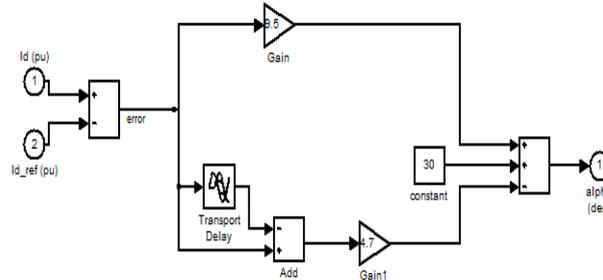
Figure 7. PD rectifier controller
