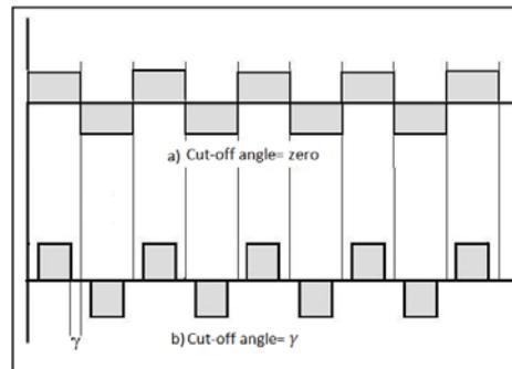
Figure 10. Cut-off angle for a phase
