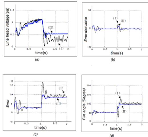
Figure 17. Performance comparison of Fuzzy-PD controller on both converters with three phase fault on load; a: line head voltage; b: error derivative; c: error; d: fire angle; (I: DC line length = 300 km; II: DC line length= 600 km)
