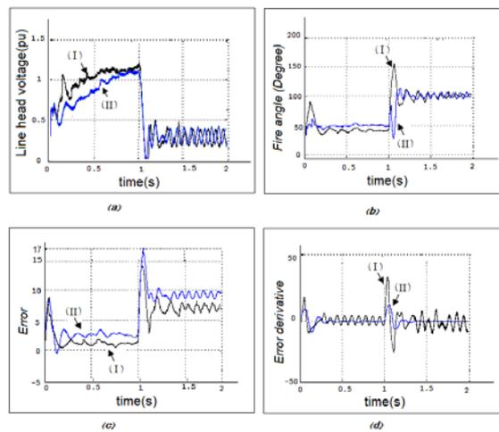
Figure 13. Comparison of performances of PD and Fuzzy-PD controllers; a: line head voltage; b: fire angle; c: error; d: error derivative; (I: PD controller on rectifier and Fuzzy-PD controller on inverter; II: Fuzzy-PD controller on rectifier and PD controller on inverter)
