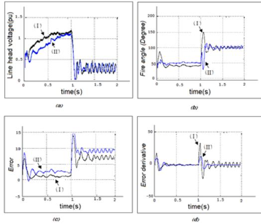
Figure 11. Comparison of performances of PD and Fuzzy-PD controllers; a: line head voltage; b: fire angle; c: error; d: error derivative; (I: PD controller on both converters; II: Fuzzy-PD controller on rectifier and PD controller on inverter)
