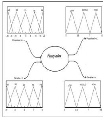
Figure 9. Membership functions for fault and derivative fault
