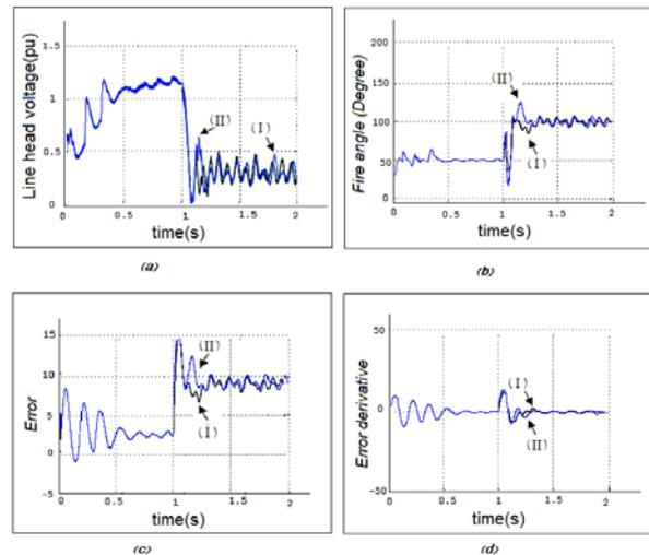
Figure 15. Performance comparison of Fuzzy-PD controller to both converters; a: line head voltage; b: fire angle; c: error; d: error derivative; (I: three phase fault on load; II: DC fault on transmission line)
