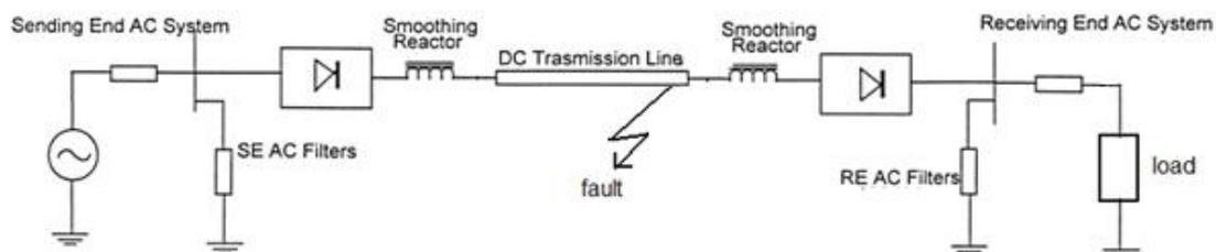
Figure 2. Single diagram of HVDC system with three-phas e fault on the DC line
