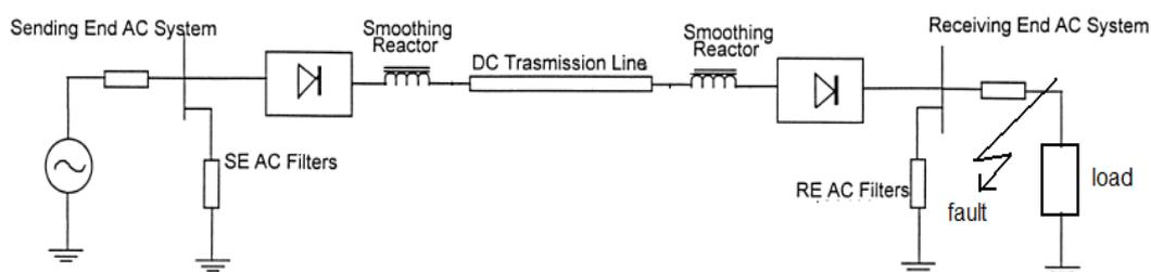
Figure 1. Single diagram of HVDC system with three- phase fault on load
